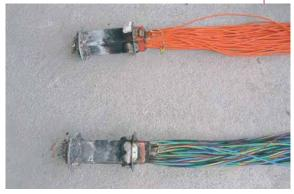
Firestop device removed after 4 hours fire test. On the exposed side all the cable disappeared. On the unexposed side, they are still perfect.
